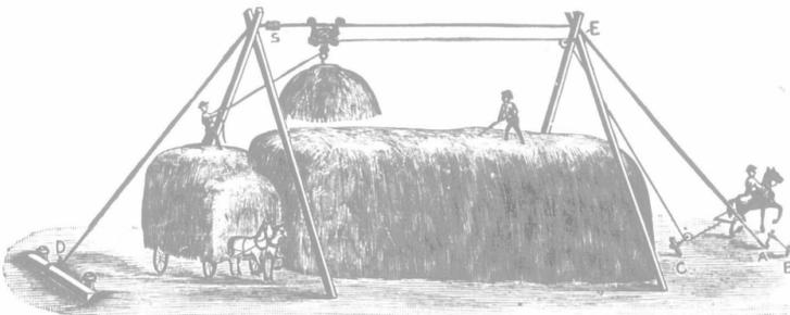
It is strong and simple, perfect working and durable, runs on 5-8 inch steel cable; uses either fork or slings, and builds any sized stack
