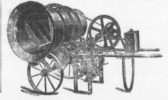
These machines are made to mix either continuously or in batches, and can be operated either by Hand, Steam or Gasov line Power.
