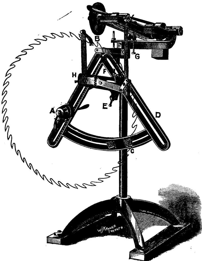
Will take saws from 6 inches to 6 feet diameter; sets the saw forward one tooth at a time automatically; sharpens any saw (rip or crosscut) perfectly, giving the teeth any desired pitch or bevel, and making all the teeth exactly alike. Will sharpen 20 teeth in an ordinary saw mill in one minute, or 100 teeth in a shingle saw in four or five minutes. The cut shows outline of mill saw 54-inch diameter.
