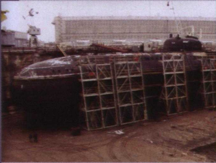
Victor III being dismantled in dry dock
