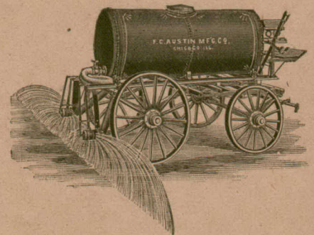
AUSTIN STEEL STREET SPRINKLER
