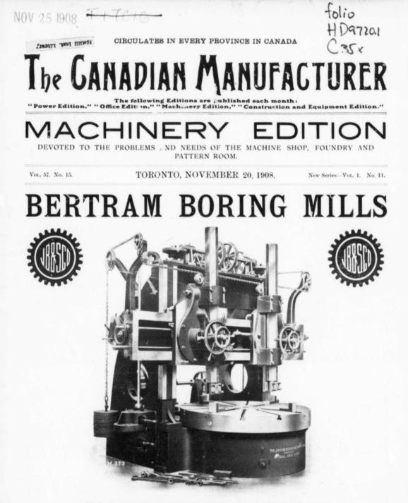
72=Inch BERTRAM HEAVY BORING and TURNING MILL
