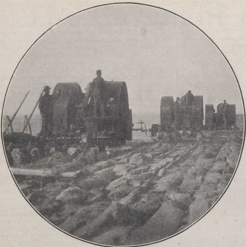
First Stage in Motor-farming: the Caravan of Gasoline Ploughs, Breaking the Prairie at the Rate of 80 Acres a Day.
