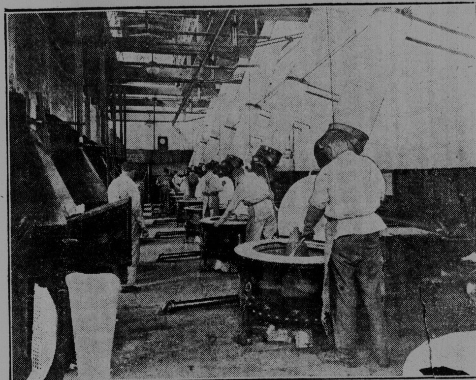
BATTERY OF NITRATING MACHINES, in which the cotton that forms the film is nitrated.
