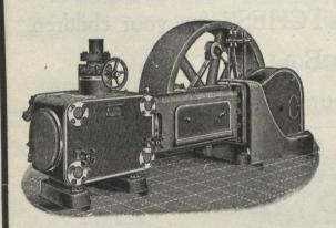
Have the Armstrong Corliss valve gear, which will operate at a higher speed than the ordinary releasing gear.
