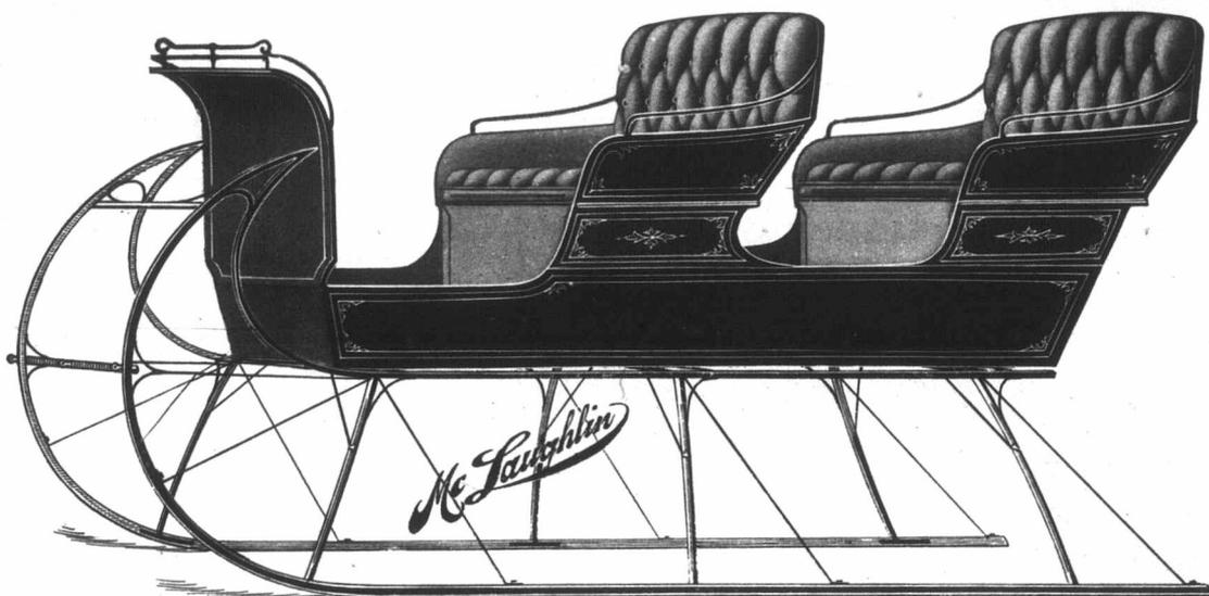
Both seats removable. Body has hardwood rail all around inside. Seats have high easy spring backs and spring cushions ; sides of seats are padded. Turned spindles on sides of body and on seat risers.
