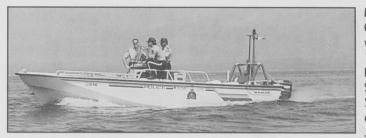
MARITIME ENFORCEMENT One of "J" Division's main weapons for enforcing Small Vessel Regulations is its Bathurst Federal Enforcement Section (FES) Guardian. The 25-foot Boston Whaler powered by twin 150-horsepower Johnson's motors, is capable of
