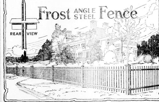
The rails are 2 inch angle steel; pickets of 3/4 inch angle steel inserted 3 inches apart through V slots in both rails and solidly rivetted; posts
