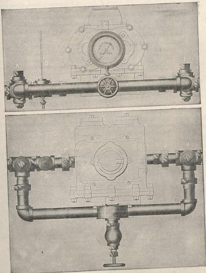
the pistons is constantly in motion, giving uniform flow of water, free from pulsation or shock. The meters are perfectly noiseless in their performance. These test meters are designed and constructed of materials uniformly affected by expansion and contraction from varying of temperatures, thus further assuring their accuracy as measuring devices.
