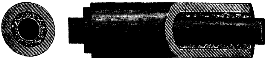
Fig. 1.—Use of Mineral Wool Inside of Wooden Collars. Plan Pursued by the New York Steam Company with its Underground Pipes.
