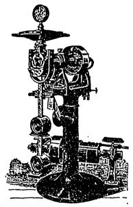
As seen from the illustration, it will be noticed that the machine consists of a frame mounted on a pillar; a shaft mounted in bearings in the frame, which shaft carries a hardened and ground pin, on which rides a pendulum provided with two special bearings. There is an arrangement for regulating the temperature by means of water, and an apparatus which registers the throw of the pendulum on a strip of paper.
