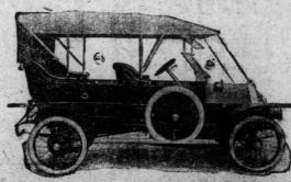
are fitted with all the latest and best improvements, including steel detachable wheels, worm or bevel drive, four forward speeds and reverse, foot accelerator, etc.
