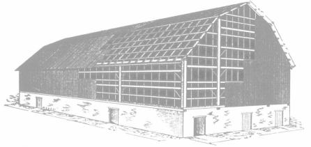
This cut shows an up-to-date Barn Construction, 40 feet x 70 feet, and the method of covering with Corrugated Sheets. The framework is light, as the corrugated sheets, when nailed in place, make the building very rigid. This drawing is made from actual plans and the barn has been built many times with splendid results.
