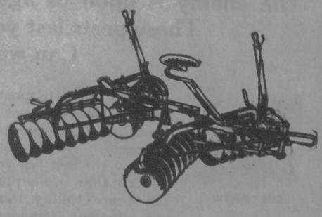
The frame on the Bissell Harrow is directly over the gangs, the draught being well back where the work is being done. The horses do not have to carry the weight of the pole, levers, braces or frame. This feature is important, and herein lies one great advantage of Bissell Disk Harrows.
