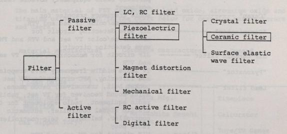
Of these, piezoelectric ceramic filters are classified by use for low frequencies or for high frequencies with major applications for TV and FM/AM radio sets.
