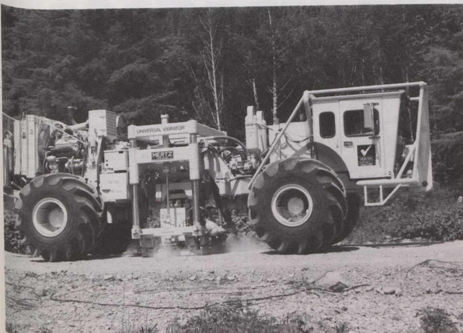
Heavy vehicle used in Lithoprobe study with metal plate that was pressed on the ground and vibrated to transmit shock waves into the ground.
