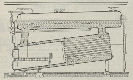
A MUMFORD Standard Internally Fired Boiler requires from 10 to 25 per cent. less fuel than a return tubular boiler.
