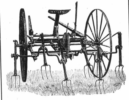
Is fitted with strong wheels, which have a double line of spokes like a bicycle.
