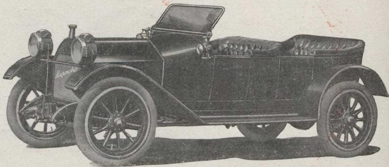
Hupmobile Long Stroke "32" Five-Passenger Touring Car—\$1,000 F.O.B. Windsor, including equipment of windshield, gas lamps, and generator, oil lamps, tools and horn. Three speeds forward and reverse. Sliding gears. Four-cylinder motor. 3½-inch bore and 5½-inch stroke. Bosch magneto. 16-inch wheel-base. 30 x 3½-inch tires. Color, Standard Hupmobile blue.
