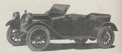
Hupmobile Long Stroke "32" Five-Passenger Touring Car-\$1,000 F.O.B. Windsor, including equipment of windshield, gas lamps, and generator, oil lamps, tools and horn. Three speeds forward and reverse. Sliding gears. Four-cylinder motor.  $3\frac{1}{2}$ -inch bore and  $5\frac{1}{2}$ -inch stroke. Bosch magneto. 106-inch wheelbase.  $30 \times 3\frac{1}{2}$ -inch tires. Color, Standard Hupmobile blue.
