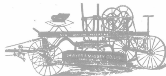
"S. & M." Steel Reversible Road Grader.
