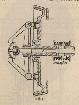
rod. In applying the effort to the toggle levers the ball-ended rod is pushed longitudinally, so that the ball end bears against the toggle levers, which force the male cone into the female cone.
