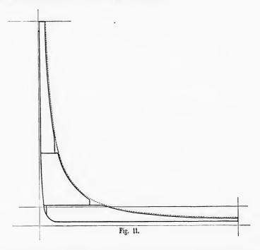
A more even division of work would be obtained by decreasing the range of pressure in the low cylinder, and increasing the range in the high. It has already been suggested that because of the relatively larger area of surface of the low cylinder a modification of this kind would probably reduce the total con-
