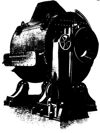
The above illustration shows our Standard "Trough" or Bisbee Converter. The shell, heads and nose are made of heavy steel plate; the ridingring of cast steel; the gear wheel is a full circle faced and bolted to a faced circular casting riveted to the head. The rack is hinged at the bottom and held in place by a cam. The wind-box is furnished with Dyblie valves.
