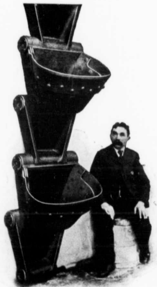
FIG. 3.—CHAIN AND BUCKET.
