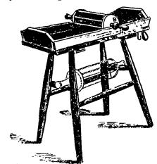
When not in use as a butter worker, the fluted roller can be placed underneath the tray out of the way (as shown in the drawing), and the tray used for other purposes, such as making up butter, &c.
