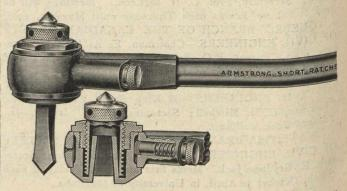
socket so as to secure a short, compact and strong ratchet drill without shortening the feed screw is the principle feature of the tool and enables the operator to drill holes in places where he could not possibly get at with the ordinary ratchet drill
