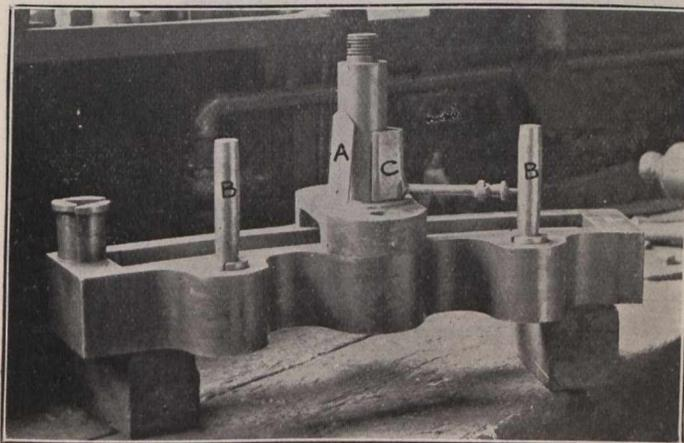
Fig. 8. Locating the Saddle Correctly on the Link.
