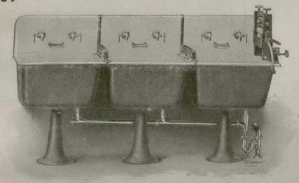
"Standard" Plate P. 1285 Porcelain Enameled Flat Rim Laundry Trays, with 12-inch Holders, Nickel-plated Union Strips with hardwood Wringer Holders, Nickel-plated Soap Dishes, Waste Plugs, Couplings and Rubber Stoppers, Nickel-plated Fuller Adjustable Flange Bibbs, Continuous Waste and Vented "S" Trap.
