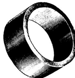
Forged, Punched and Rolled from a Solid Chrome Steel Ingot
