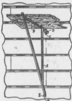
Small Grappler as used between Vertical Joints of Brickwork.
