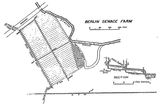
the different buildings is collected in a large tank constructed of brick and lined with cement, having a capacity of rather more than 100,000 gallons. From the tank the sewage is pumped by a six-inch rotary pump to the filtration area, through an eight-inch spiral riveted steel pipe comprises about four acres, laid out in eighteen parallel ditches eight feet wide plane. The sewage is conveyed to these by an eighteen-inch vitrified channel pipe
