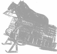
The McGILL MONARCH TREAD POWERS are The McGILL MONARCH TREAD POWERS are the best general-purpose Farm Powers on earth, and are the only Powers made having Angle Steel Track, Cold Rolled Steel Shaft, 7-inch Travellers, Solid Maple Lags, with Brake entirely independent of Band Wheel. A Patent Governor or Speed Regulator with each Machine,
