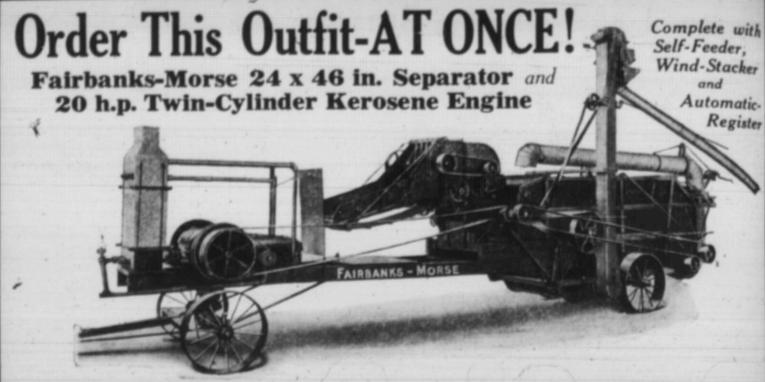
For simplicity, correct design and efficient work under all conditions you cannot buy a better combination thresher. The Fairbanks-Morse gets all the grain. Sills of seven-inch channel steel, with five-inch channel girts, give perfect rigidity. Herey steel body, double-bar cylinder, long bearings and heavy shafting every feature that makes for good work and durability is found in our separators.
