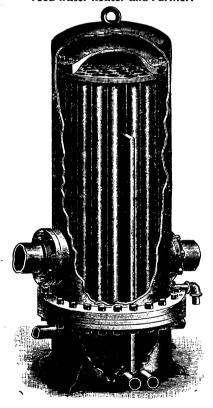
GREAT EFFICIENCY, SIMPLICITY OF CONSTRUCTION and LOW COST. Has a Cast Iron shell, which will never wear out, with seamless drawn brass tubes expanded into tube-plates at top and bottom, with double blow-off.
