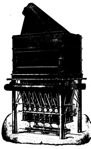
We illustrate herewith a 42 inch by 120 inch steel water jacketed copper smelting furnace which embodies all the latest improvements in copper smelting.
