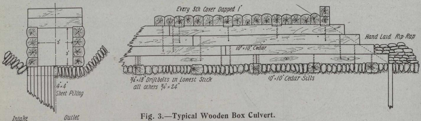
Fig. 3.—Typical Wooden Box Culvert.
