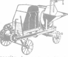
Two machines in One.—It mixes any kind of Concrete or Mortar, and does any kind of hoisting at the same time. Built in two sizes.
