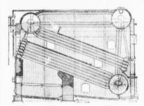
Free Expansion of Tubes, Perfect Water Circulation, Dry or Superheated Steam, Half the usual number of Handholes.
