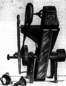
This is our No. 2 Grinder, with elevator suitable to be run by tread power or sweep power. Has divided hopper for crushing and grinding corn on the cob as well as small grain. Elevator attached as above when desired. Please notice that it is provided with a double discharge spout and switch board, so that one sack can be removed while the other is filling. Send for catalogue. We also manufacture Tread Powers, Threshers, Feed Cutters, Hay Presses, Circular Saw Machines, etc., etc.
