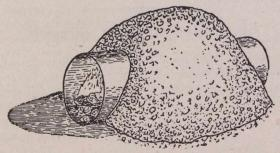
Defective cast iron water pipes are quite suitable for this work. Frequently we have seen sheets of steel or wrought iron used, but when they become heated, they warp and cave in, and thus are not so suitable as the cast-iron pipe.
