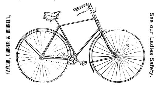
THE POPULAR RAGLAN SAFETY, built especially for Canadian Trade. The finest Wheel for the price, and guaranteed for a year. Frame of Weldless Steel Tubing and Steel Stampings, Ball Bearings throughout, Ball Socket Head, Cushion Fire, Garford Saddle. Price, \$85.00. Special.
