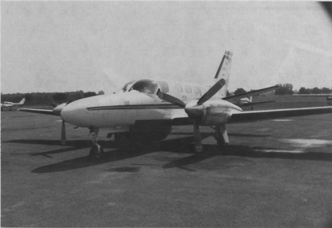
Figure 4. Twin-engine Cessna Conquest equipped with a synthetic aperture radar. The Conquest is a cost-effective platform which delivers the altitude, range and speed capabilities required to operate a SAR. The Conquest provides a service ceiling of about 11,275 metres and has a maximum range of about 4,000 kilometres when flying at 10,000 metres. The aircraft would also make a good platform for an infrared linescanner and/or a camera system. (Courtesy Intera Technologies Ltd.)
