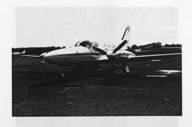
Figure 20. Twin-engined Cessna Conquest equipped with synthetic aperture radar. The Conquest is a cost-effective platform which delivers the altitude, range and speed capabilities required to operate a SAR. The aircraft would also make a good platform for an infrared linescanner or mapping camera. (Courtesy Intera Technologies Ltd.)
