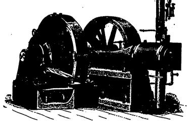
HE above cut represents a ROBB-ARMSTRONG Engine direct connected with dynamo. Simple, Tandem, or Cross Compound Engines may be used combined with any standard type of Dynamo.
