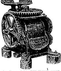
IMPLEMENTS FOR THE MANUFACTURE of syrup and sugar from Sorghum.—Crushers with three cylinders.—Carbonic acid gas engines, Racking-tubs Livaporators. Thormometers. Areometers —FOR SUGAR. Vacuum pans, Crysta'nzing boilers; Mixers; Contrilugals, &c.
